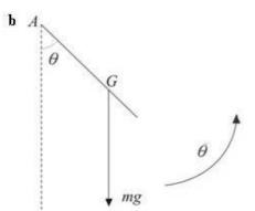
Let A be the vertex of the cone and G the centre of mass of the cone.
