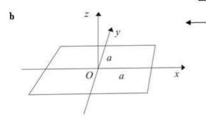
Let O be the centre of the plate, Ox and Oy be axes parallel to the sides of the square and Oz be the axis through O perpendicular to the plate, as shown in this sketch. The question asks you to find the moment of inertia about Oz.
