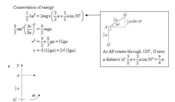
Let the magnitude of the vertical component of the force acting on the rod at A immediately after the impact be Y.
