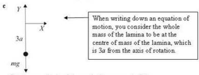
Let the magnitude of the vertical component of the resultant force of the axis PQ on the flap, as it reaches the vertical position be Y.
