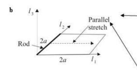
Let  $l_1$  and  $l_2$  be axes along two of the sides of the square and  $l_3$  be the axis through the corner perpendicular to  $l_1$  and  $l_2$ , as shown in this sketch. The question asks you to find the moment of inertia about  $l_3$ .
